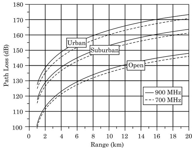
**Fig. 2.18** Path loss predictions with Hata propagation model for a mid-sized city [Base antenna – 30 m, Mobile antenna – 1 m]
