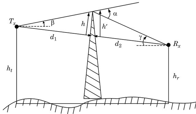
(b) Knife-edge diffraction geometry when the transmitter and receiver are not at the same height. Note that if  $\alpha$  and  $\beta$  are small and  $h \ll d_1$  and  $d_2$ , then  $h$  and  $h'$  are virtually identical and the geometry may be redrawn as shown in Fig. 2.7c.
