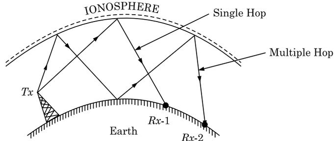
**Fig. 2.14** Sky wave propagation through Ionosphere
