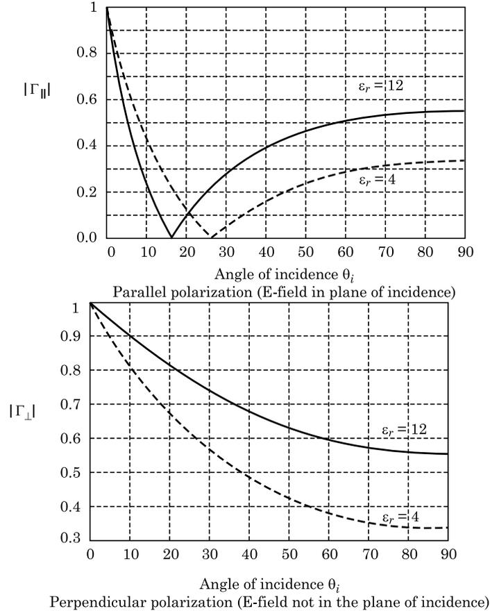
**Fig. 2.6** Reflection coefficients vs angle of incidence
