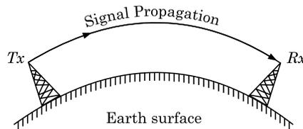
**Fig. 2.13** Ground Wave Propagation ( $< 2\text{MHz}$ )
