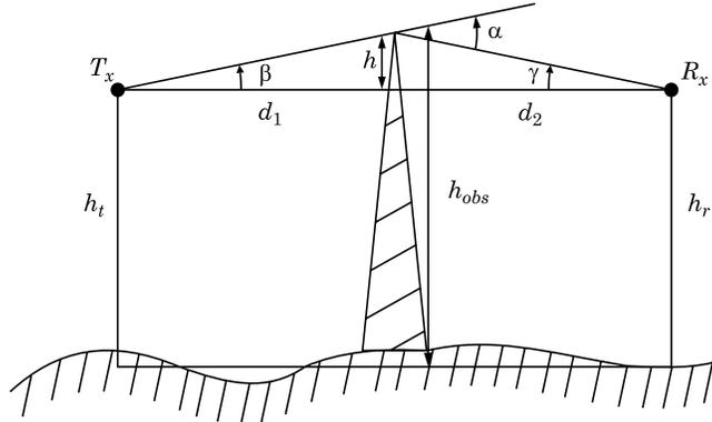
(a) Knife-edge diffraction geometry. The point  $T_x$  denotes the transmitter and  $R_x$  denote the receiver, with an infinite knife-edge obstruction blocking the line-of-sight path.
