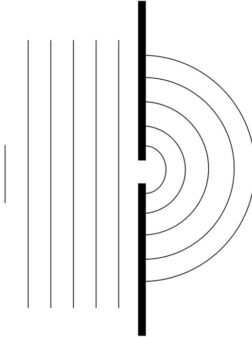
**Fig. 2.7** *Plane passing through a slit left to right*
