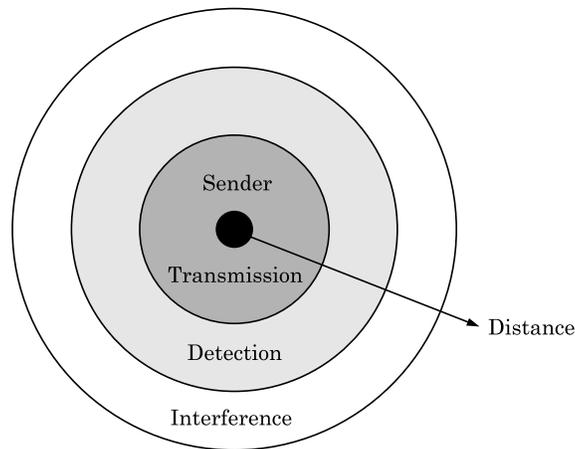
**Fig. 2.1** *Ranges for transmission, detection and Interference of Signals*
