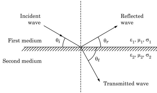
$\theta_i \rightarrow$  angle of incident wave with the plane
