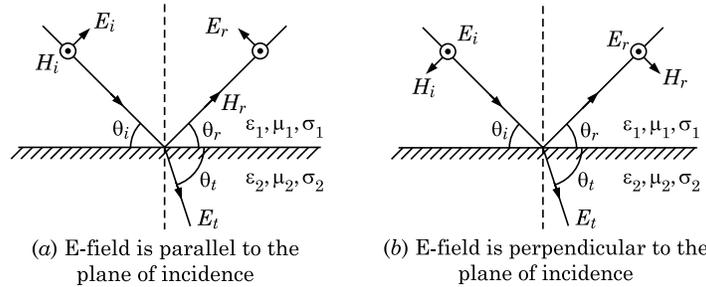
**Fig. 2.4** Reflection coefficients between two dielectric
