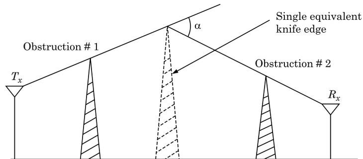
**Fig. 2.12** Multiple Knife-edge diffraction model
