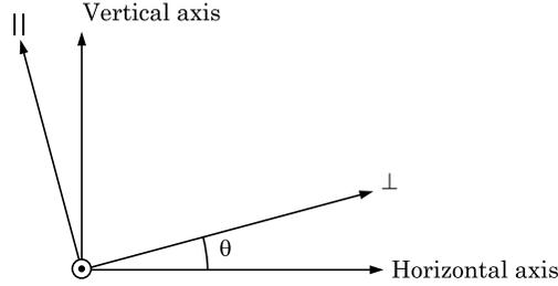
**Fig. 2.5** Axis of orthogonally polarized components. Wave is propagating out of the page (toward the reader)
