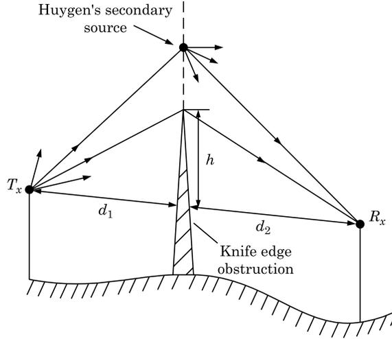
**Fig. 2.10** Knife-edge diffraction model geometry. The receiver  $R_x$  is located in the shadow region
