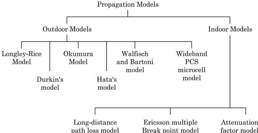
**Fig. 2.17** Classification of Propagation Models.
