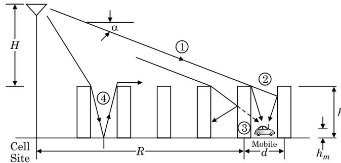
**Fig. 2.19** Propagation geometry of Walfisch and Bertoni's Model.
