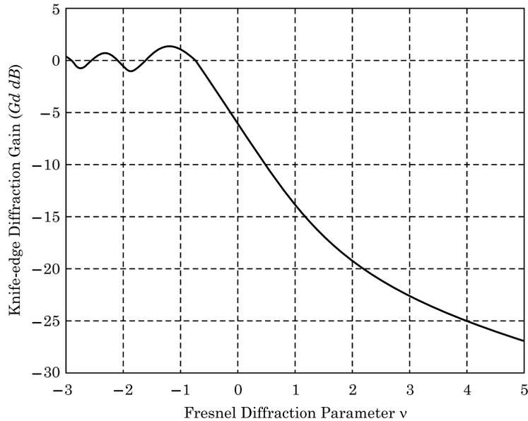
**Fig. 2.11** Graphical representation of diffraction gain as a function of Fresnel diffraction parameter
