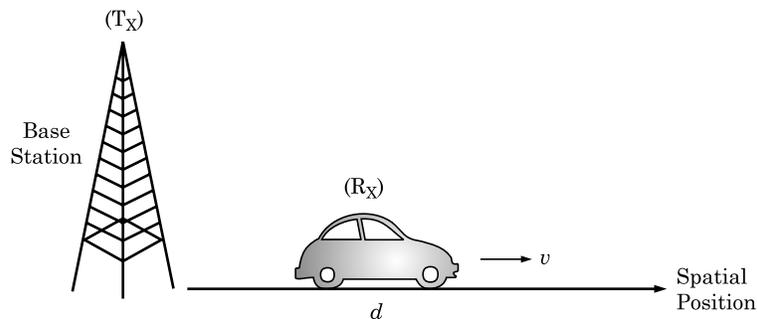
**Fig. 3.7** *The mobile radio channel as a function of time and space.*
