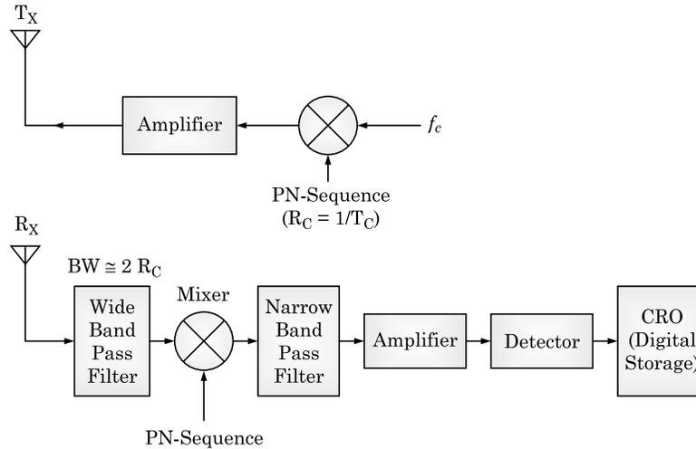
**Fig. 3.5** Block representation of spread spectrum shielding correlator measurement technique.
