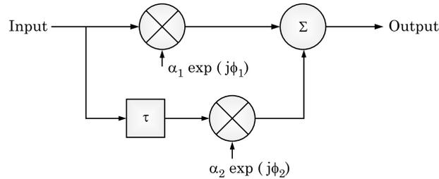
**Fig. 3.10** *Two ray rayleigh fading model*
