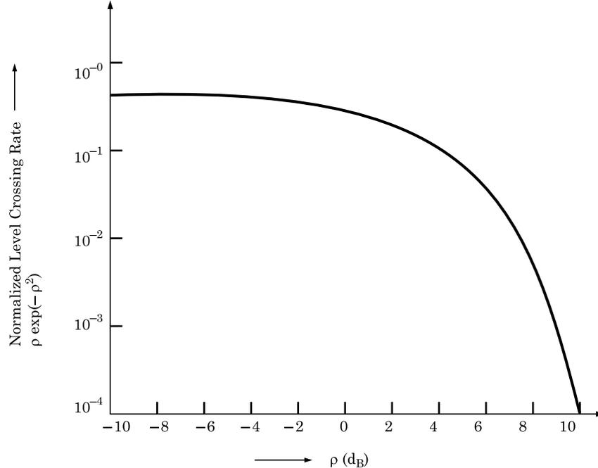
**Fig. 3.12** The normalized level crossing rate of flat Rayleigh Fading channel.
