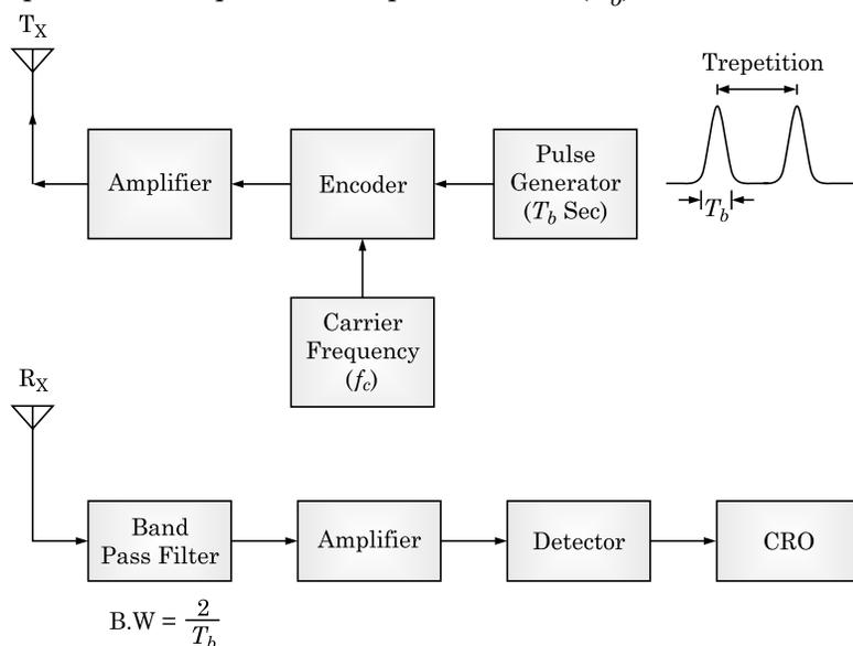
**Fig. 3.4** Direct Pulse Measurement technique.
