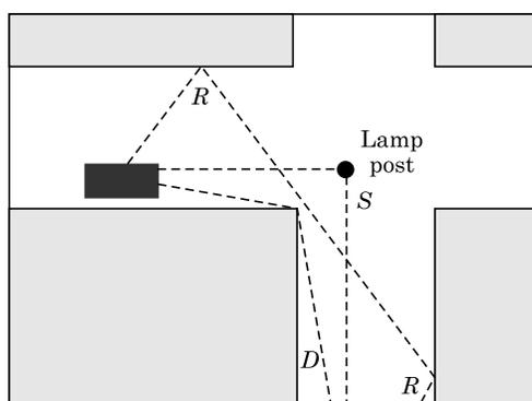
**Fig. 3.2** Three Important Propagation Mechanism: Reflection (*R*), Scattering (*S*), Diffraction (*D*)
