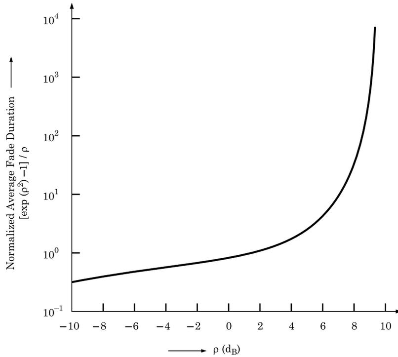
**Fig. 3.13** The normalized average fade duration of the flat Rayleigh Fading channel.
