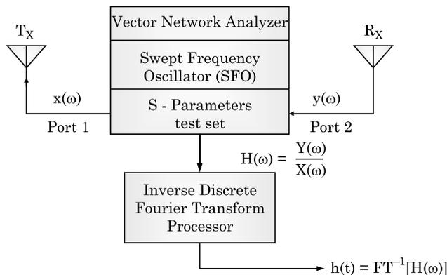
**Fig. 3.6** Swept frequency measurement technique to measure channel impulse response in frequency domain.
