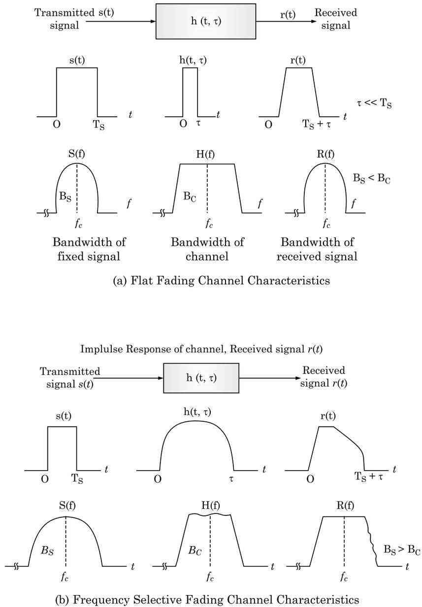
**Fig. 3.9** Different small scale fading characteristics based on multipath time delay spread.
