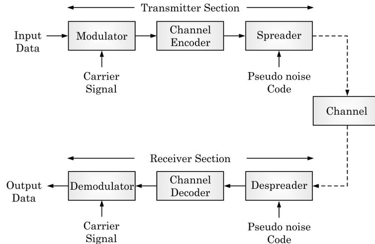
**Fig. 4.2** Block diagram of Spread spectrum digital communication system.
