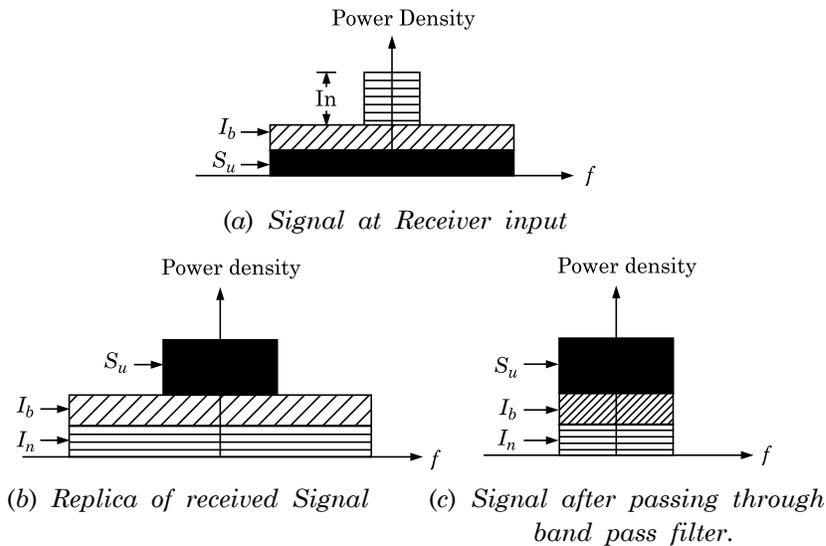
**Fig. 4.5** Despreading of a wideband signal.
