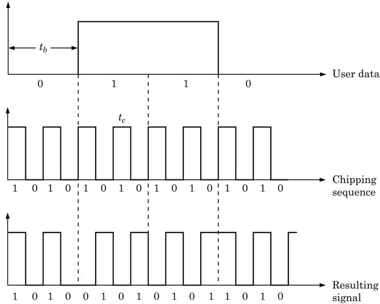
**Fig. 4.7** Spreading the signal with DS-SS.
