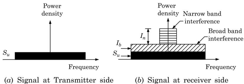
**Fig. 4.4** Interference added during transmission.
