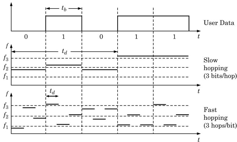
**Fig. 4.10** *Slow and Fast frequency hopping.*
