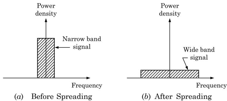
**Fig. 4.3** Spreading of a narrowband signal.
