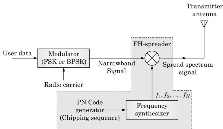
**Fig. 4.11** *FH-SS Transmitter.*
